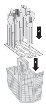
To make the removal of cutlery easier, on some dishwasher models it is possible to open the cutlery rack. If you use the grid insert then the cutlery rack cannot be opened.
